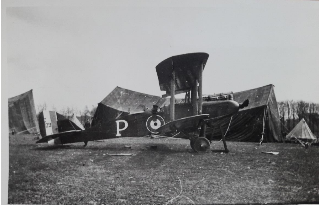
Airco DH9 C6109, which Harold Wild was flying when he was shot down and killed on 16 th June 1918. The DH9 could carry up to 209kg of bombs and was equipped with one forward firing Vickers machine-gun and one or two rear-firing Lewis guns on a ring mounting. It cannot be known for certain whether the photograph shows Harold Wild at the controls (JM Bruce/G.S. Leslie Collection)
